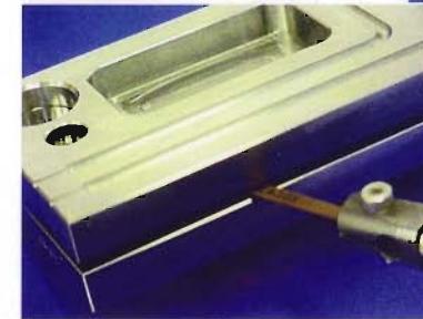
Precise polishing of ribs
