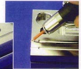
Precise polishing of sub-gates
